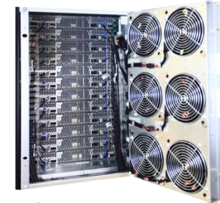
Redundant Power Supplies & Fan Modules
