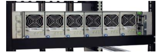
5 + 1 Redundant Power Supplies
