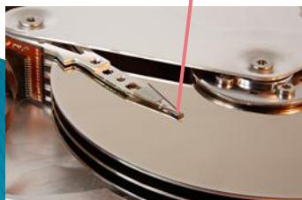
HDD was realized the significant growth by GMR/TMR Head that was the breakthrough for the SNR limit.
