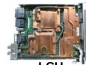
LCU (Liquid Cooling Unit)
